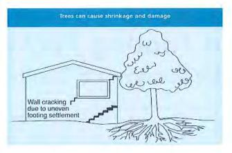
As the weather pattern changes and the soil begins to dry out, the external footings will be first affected, beginning with the locations where the sun's effect is strongest. This has the effect of lowering the external footings. The doming is accentuated and cracking reduces or disappears where it occurred because of dishing, but other cracks open up. The roof lines may become convex.
